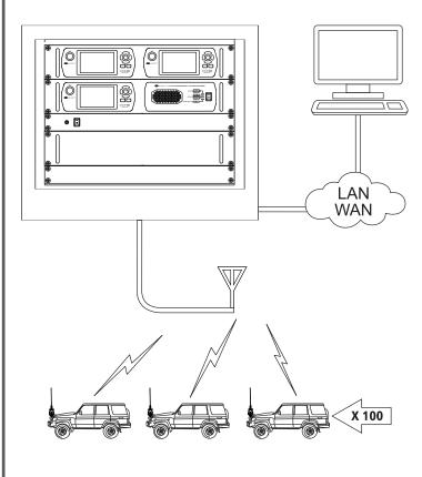
This scenario has 100 mobile transceivers, each with 3 channel programmed for GPS Push transmission. Each GPS Push transmission in this scenario takes approximately 10 seconds (assuming an antenna with memory tune is fitted).
