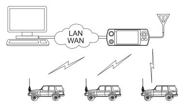
This scenario has 3 mobile transceivers, each with 6 channels programmed - 4 for voice transmission and 2 exclusively for consecutive GPS Push transmissions.
